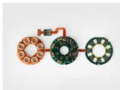
8-layer flex-rigid multilayer • assembled with coils
