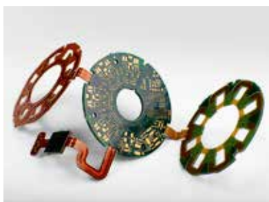
8-layer flex-rigid multilayer • filled blind holes in rigid- and flexible areas • separated flex layers with coverlay foil
