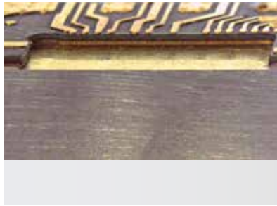
Heat sink solution • 6-layer PTFE/FR4 • conductive adhesive CF 3350-004 • aluminium heat sink goldplated • optimal heat dissipation
